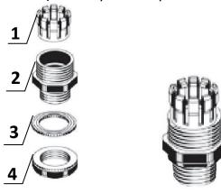
3. The pre-assembled network and grounding cables to pass through the waterproof cover set as shown.
