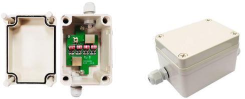
SP006PHO is a high quality surge protection device which special design to protect outdoor POE/Network equipment from lightning. The product is enclosed in a IP66 outdoor housing which could be easily mounted on a wall or a pole. It supports data transmission up to 1 Gigabit and POE device up to 90W.
